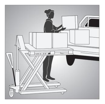
Figure 35 - Scissor pallet jack open pallet
