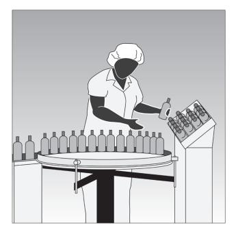
Figure 39 – Turntable for buffering products
